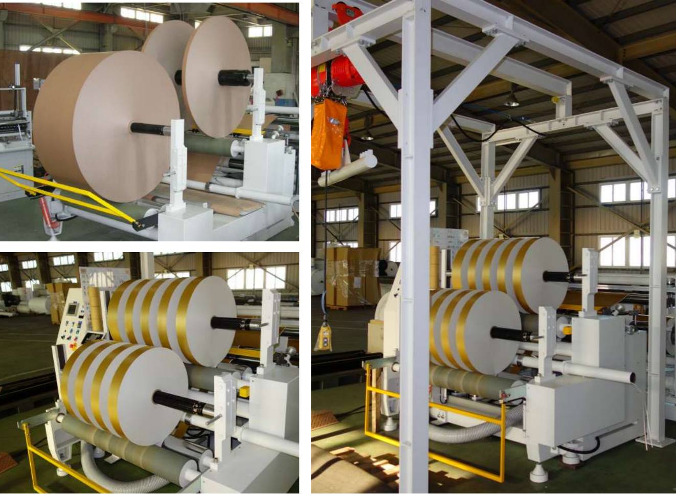
Ref : The EG-2L Duplex Shaft Surface Winding Slitter : A rather manual model with great capability of handling large paper rolls.
