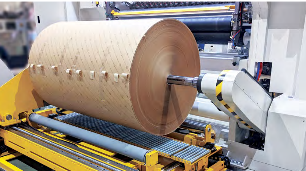
EG-8002 Series Duplex Shaft Center-Winding Slitter Rewinder installed at a customer's factory in Germany
