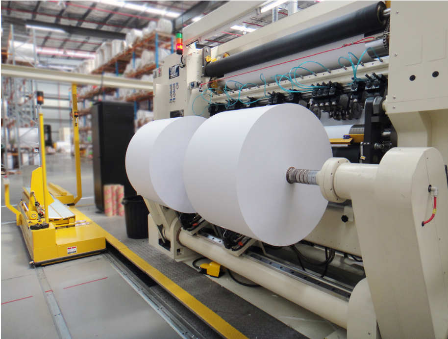
A slitter rewinder installed for a world-leading label company. (EG-8002 series)
